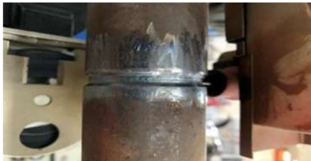
The formation of root welding
